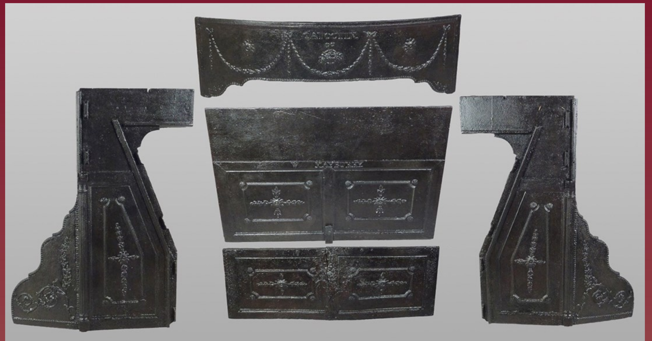
Figure 1. Five plates from the Catoctin Furnace Historical Society's Franklin stove, with manufacturing information and molded decoration, after conservation.
